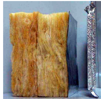
Figure 34: Vacuum insulation material panel compared to mineral wool panel of the same thermal resistance. ( www.vip-bau.ch )
