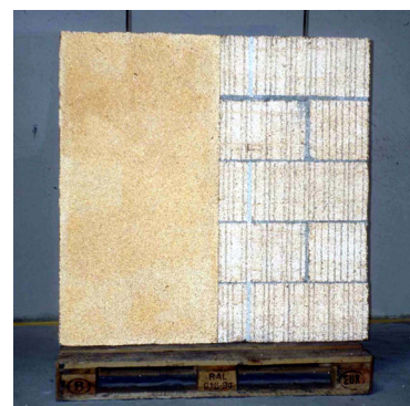
Figure 33a: Application of glass-bubble plaster compared to conventional plaster on brick.
